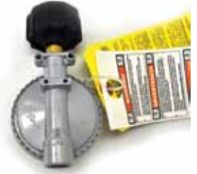
658 100k Btu LP pressure regulator 3/8" x 3/8", 4"-12" water column
