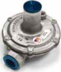
770-150 150k Btu pressure regulator Natural Gas : 5 psi input Liquid Propane: 2 psi input 1/2"x1/2", 4"-12" water column
