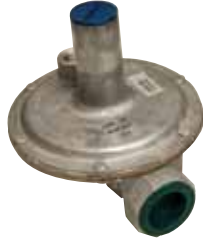
770-300 300k Btu pressure regulator Natural Gas : 5 psi input Liquid Propane: 2 psi input 1"x1", 4"-12" water column
